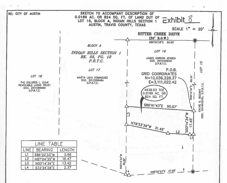
1. THE COORDINATE SHOWN HEREON IS BASED ON THE TEXAS STATE PLANE COORDINATE SYSTEM, CENTRAL ZONE, NAD83 (CORS96) DATUM AND WAS ESTABLISHED BY GPS OBSERVATION. THE BEARINGS SHOWN ARE GRID BEARINGS. THE COMBINED GRID TO SURFACE SCALE FACTOR IS 1.00005. ALL DISTANCES SHOWN ARE SURFACE DISTANCES.
