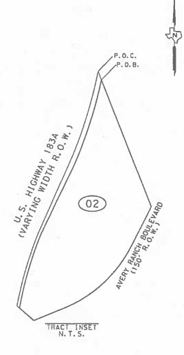
BASIS OF BEARINGS IS THE TEXAS COORDINATE SYSTEM OF 1983, CENTRAL ZONE NAD 83/2011. ALL COORDINATES AND DISTANCES SHOWN MEREON ARE SURFACE AND MAY BE CONVERTED TO GRID BY USING THE SURFACE ADJUSTMENT FACTOR OF 1.00012. UNITS: U.S. SURVEY FEET.
