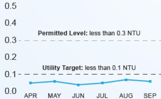
Measured turbidity "cloudiness of water" is the indicator of the effectiveness of our filtration systems. Our target is to keep treated drinking water turbidity level at 0.10 Nephelometric Turbidity Unit (NTU) or less.
