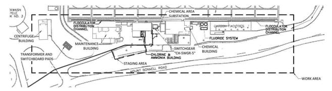
The buildings under scope for this project are the Chlorine and Ammonia (CLAB) building, the Maintenance Building, the chemical building and the Centrifuge building. The project includes replacement of all natural gas HVAC systems and water heaters with electric heating systems.
