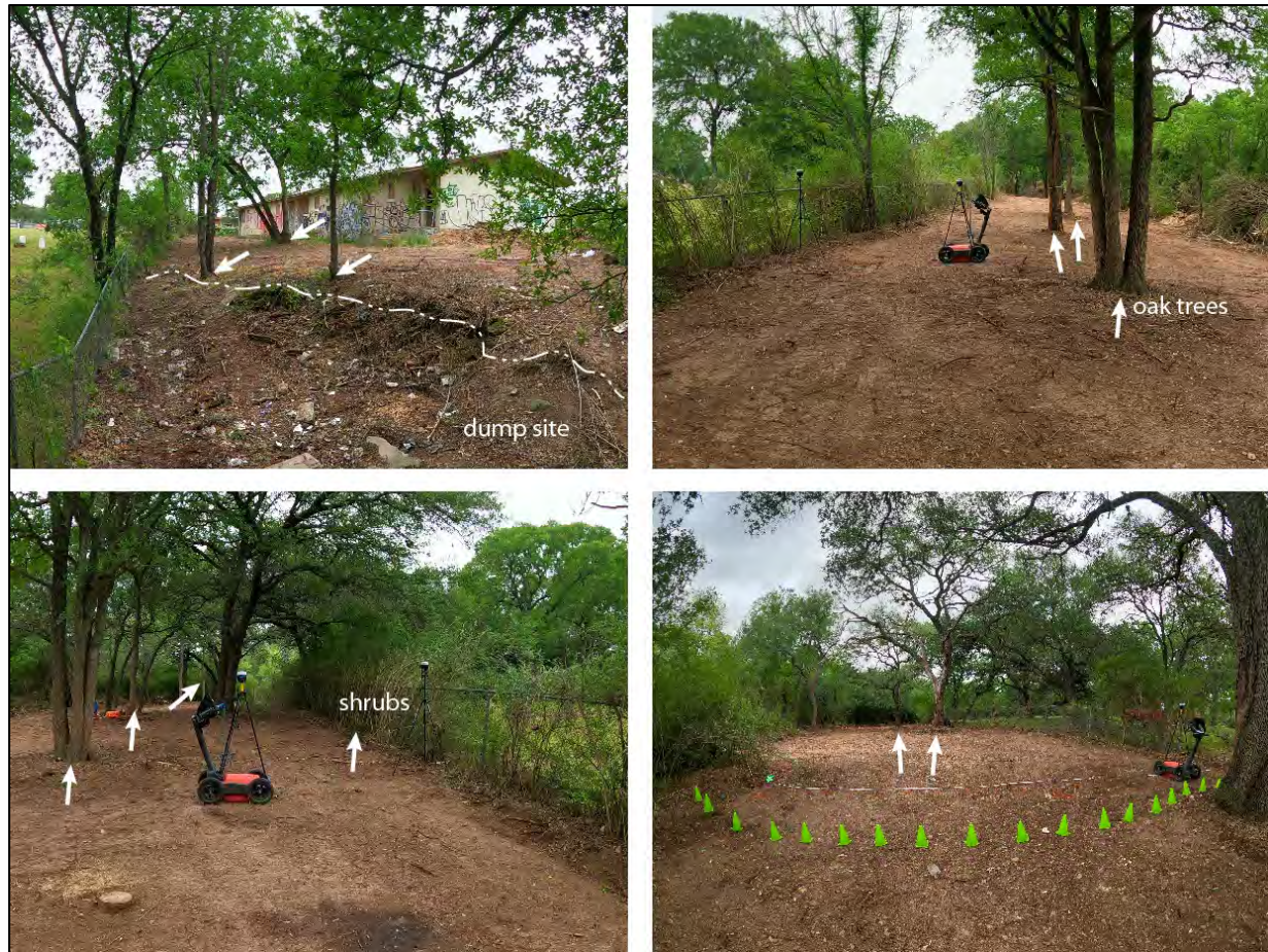
Figure 4. Examples of physical obstacles encountered by the GPR unit during the survey in Area 1 and Area 2. The obstacles cause significant delays in data acquisition, make data processing more demanding, and yield data gaps.
