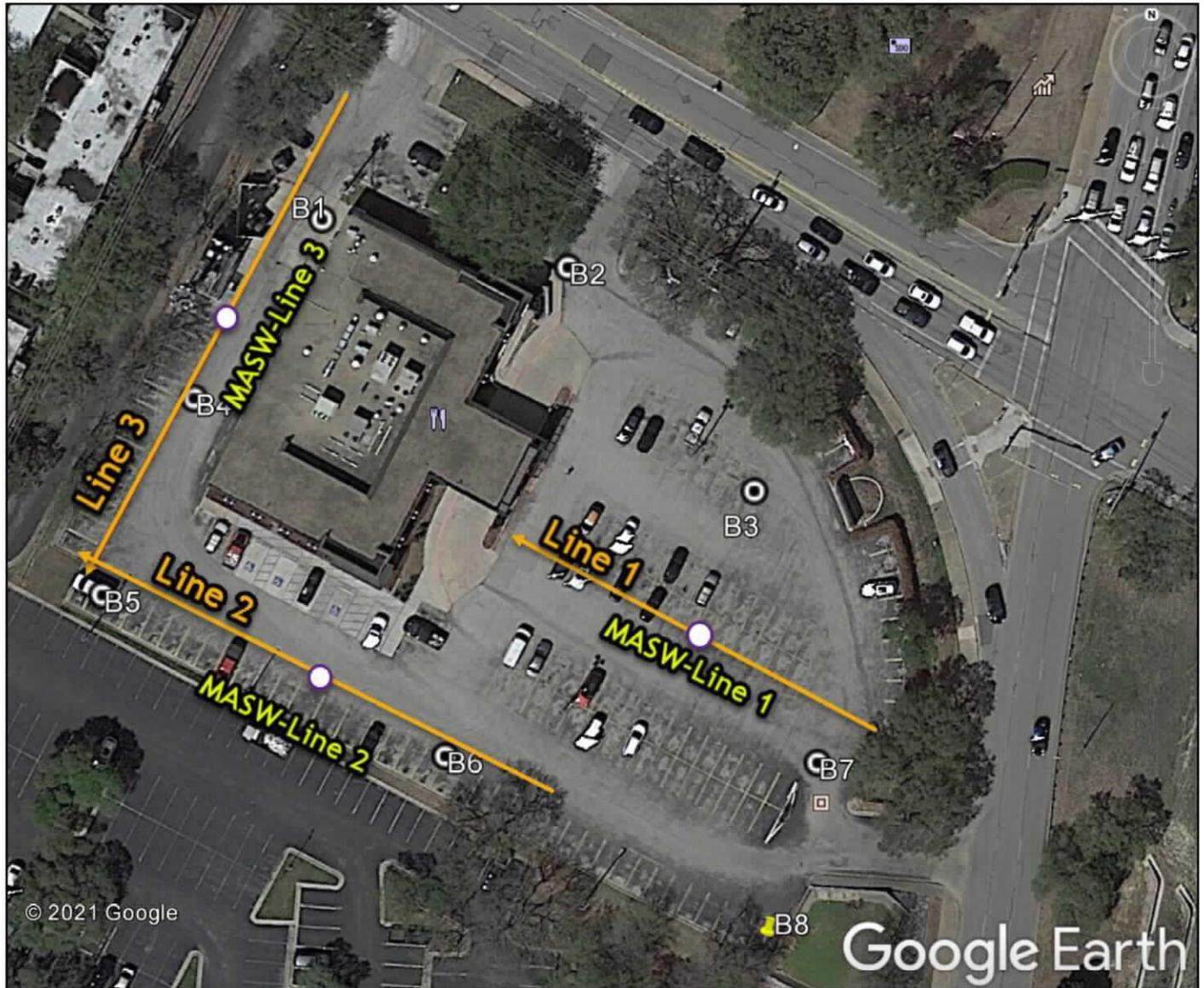
Figure 3: The location and orientation of Seismic Refraction Tomography survey lines
