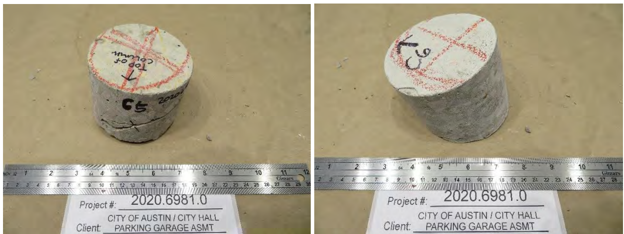
Figure 2. As-received Core C5 and C6, with Core C5 broken near the bottom.
