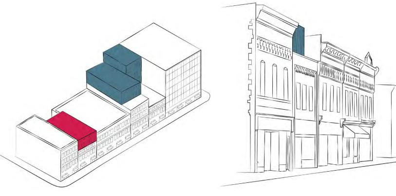
Set back additions from the front wall of the historic building at least 20' to preserve the appearance of the existing massing. The addition in red does not meet this standard.
