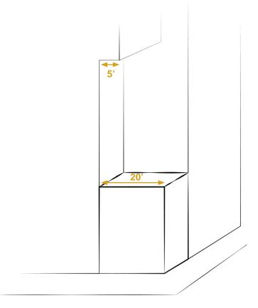
Standard 2.4 provides minimum requirements for cantilevered additions. An addition must respond to, prioritize, and be subordinate to the historic building, even if that means greater setbacks and vertical spacing.
