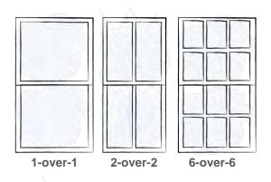
Above: The window type and number of lites, or panes of glass, in a window speak to a building's construction period and architectural style. Early windows are typically 1-over-1 or 2-over-2 double-hung wood-sash windows; the 6-over-6 lite pattern appeared in the 1930s and 40s. Sometimes window screens added ornamentation by making windows appear to contain more lites.
