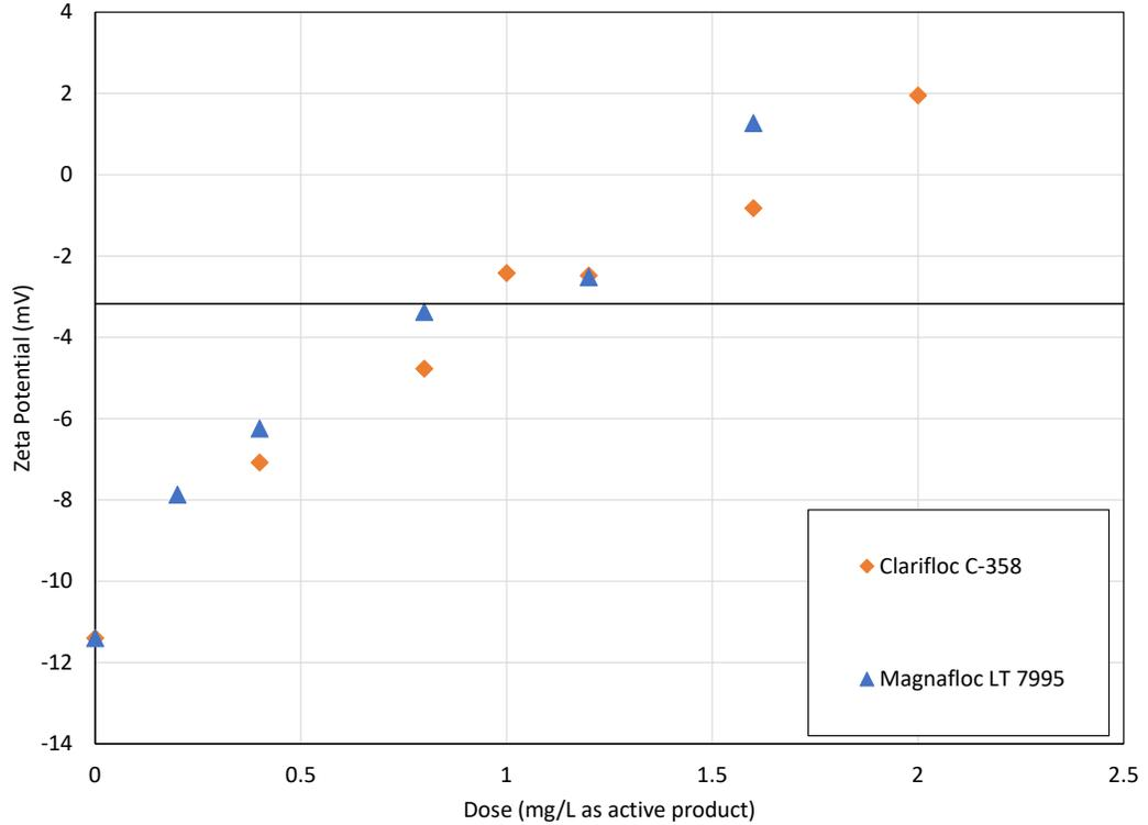
Figure F.2 Impact of PEC Dose on Zeta Potential in Typical Water
