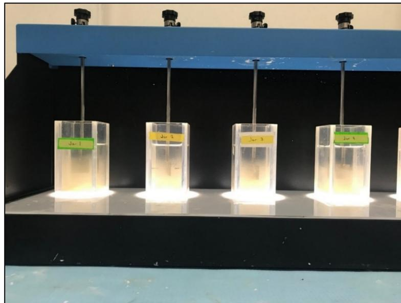
Figure 31 Image of Solids Settling in 200-mL Jars with CO<sub>2</sub> Doses Increasing (left to right) from 0 to 65 mg/L
