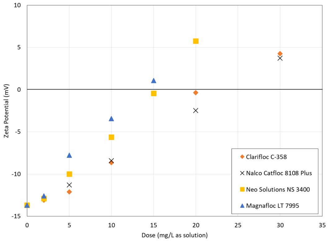
Figure 8 Impact of PEC Dose on Charge Neutralization
