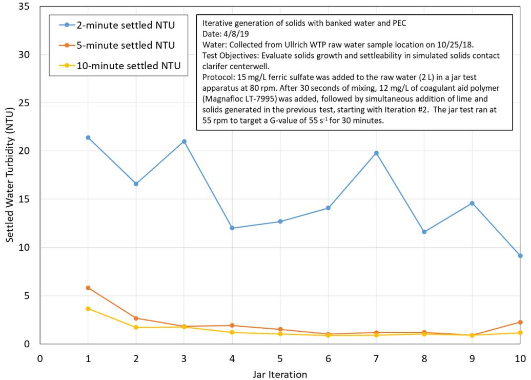
Figure 23 Iterative Generation of Solids with 0 mg/L PEA
