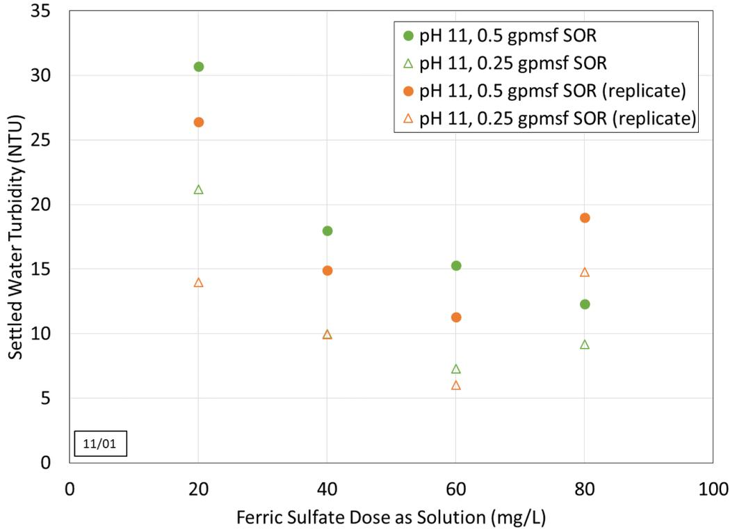
Figure 15 Impact of Ferric Dose on Settled Turbidity - 11/1/18
