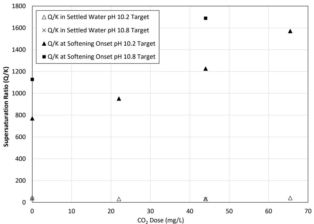
Figure 29 Impact of Carbon Dioxide Addition on CaCO<sub>3</sub> Saturation
