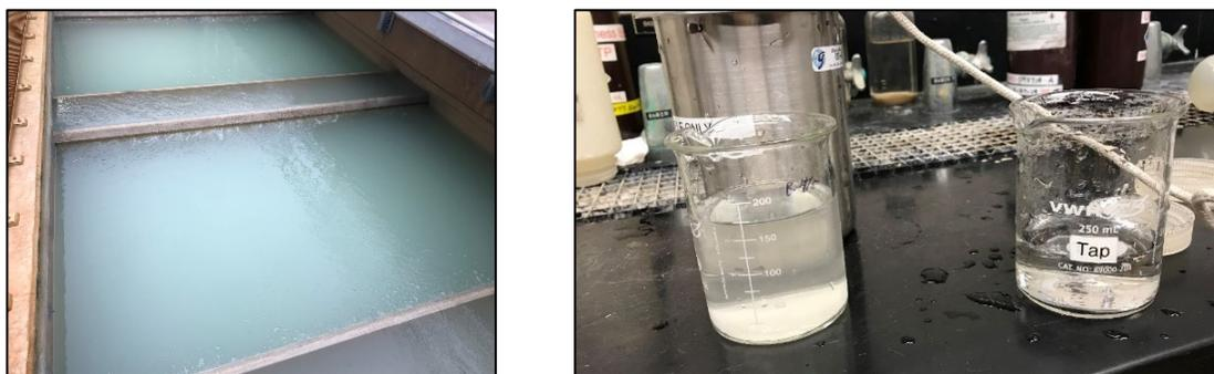
Figure 10 Precipitation in Filter Supernatant
