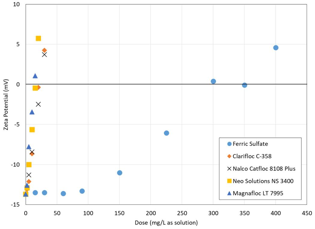
Figure 7 Zeta Potential Titration with Ferric Sulfate and Cationic Polymers (PEC)
