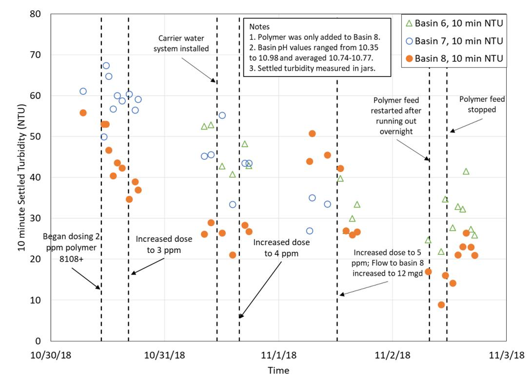
Figure 32 Demonstration-Scale Polymer Addition Timeline: Mixing Well Solids Settled Turbidity
