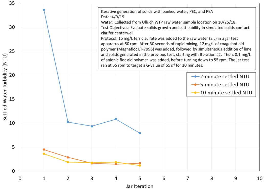
Figure 25 Iterative Generation of Solids with 0.1 mg/L PEA
