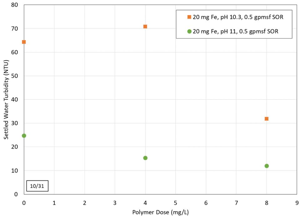
Figure 25 Impact of Offsetting Ferric Sulfate with Nalco 8108+ PEC (Low Range) on Settled Turbidity
