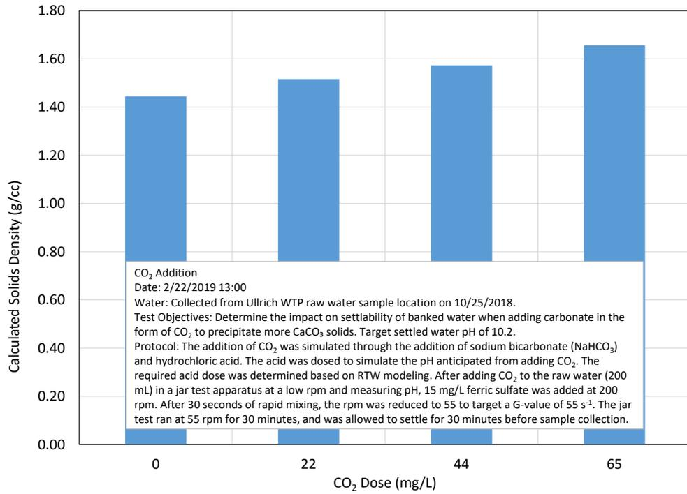
Figure 30 Impact of Carbon Dioxide Addition on Calculated Solids Density<sup>5</sup>
