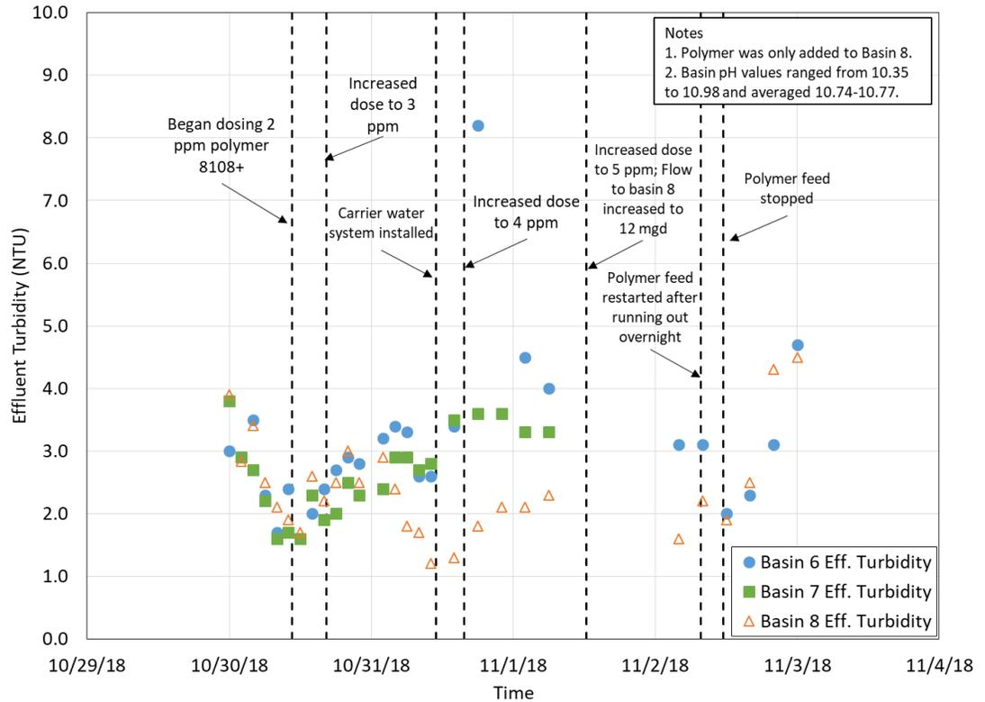
Figure 33 Demonstration-Scale Polymer Addition Timeline: Settled Water Turbidity
