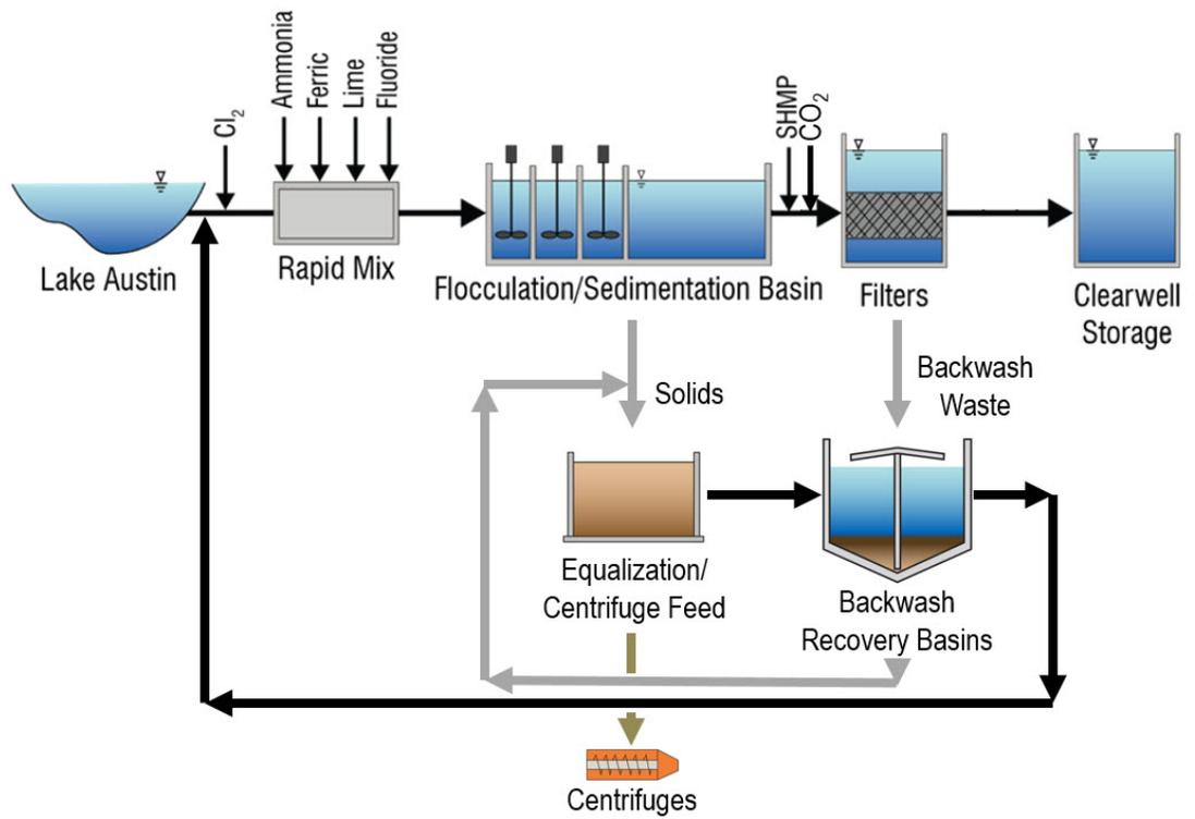
Figure 9 Process Flow Diagram for Davis WTP (120 mgd)
