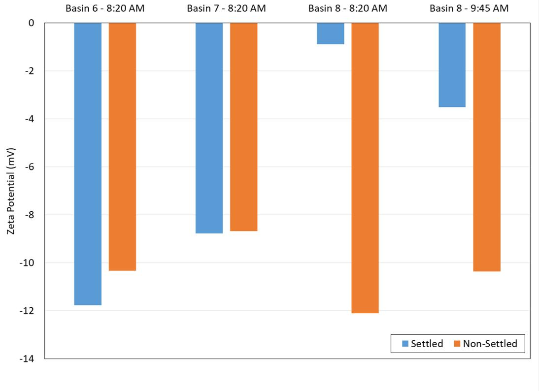
Figure 34 Impact of Demonstration-Scale Polymer Addition on Zeta Potential
