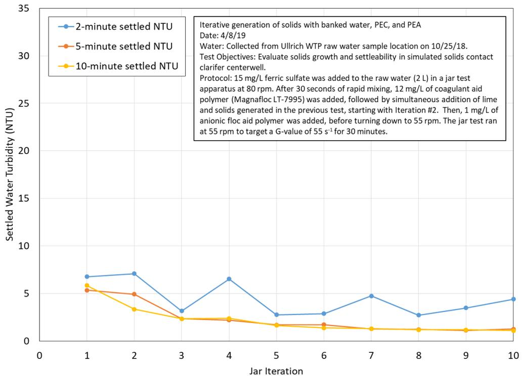
Figure 24 Iterative Generation of Solids with 1 mg/L PEA
