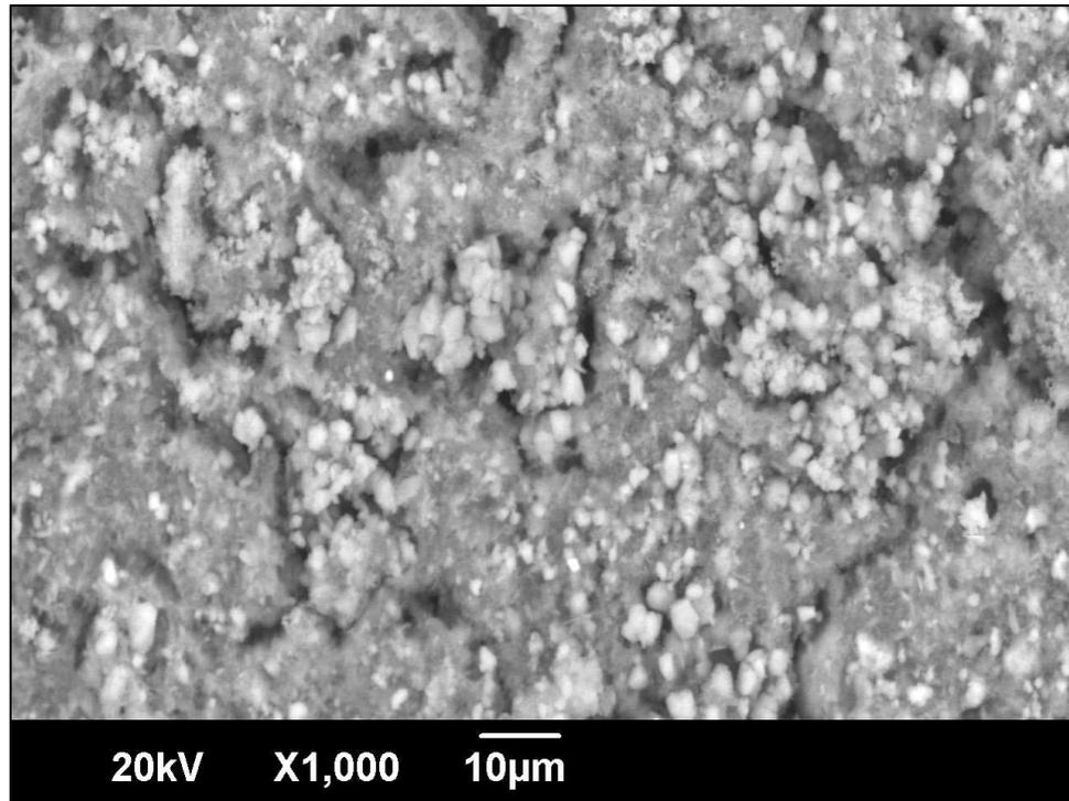
Figure D.8 SEM Image of Solids Produced with Banked Water Softened at pH 10.2 with 15 mg/L Ferric Sulfate and 12 mg/L PEC (Solids Generation Iteration #10)
