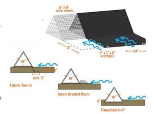
**Mulch Socks:** A mulch sock consists of material encased in a 12" or 18" diameter tube of mesh and provides an environmentally-sensitive alternative to silt fencing.
