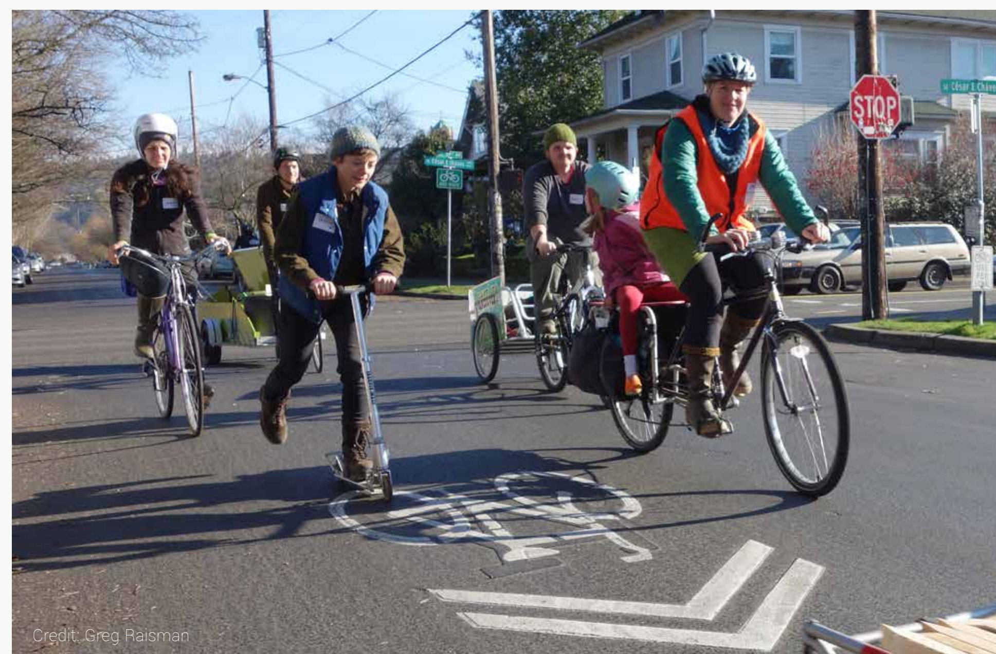
Example of a shared lane marking, aka “sharrow,” on a neighborhood bikeway in Portland, Oregon.
