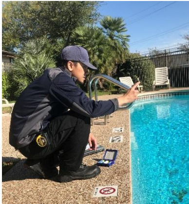
Khanh Le, Registered Sanitarian reading chemical results from pool sample during an inspection.
