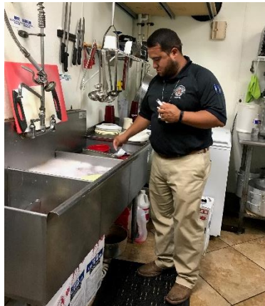
Anthony Sandoval, R.S. performs a sanitizer concentration test using chlorine test paper in a ware wash sink.
