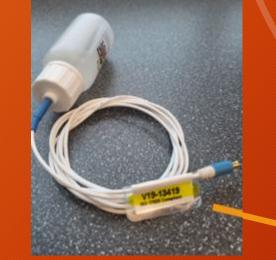
DATA LOGGERS WILL HAVE AN EQUIPMENT ID NUMBER LOCATED ON THE BACK, ALWAYS VERIFY EQUIPMENT ID TO THE NUMBER ON THE PROBE'S CORD TO ENSURE THEY READ THE SAME BEFORE CONNECTING THE CORRECT CORD BEFORE POWERING ON.
