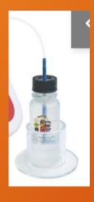
PLACE PROBE CENTER OF UNIT ENSURING THAT PROBE CORD IS RUN TO THE OUTSIDE OF THE UNIT NEXT TO THE PLASTIC HOLDING CRADLE
