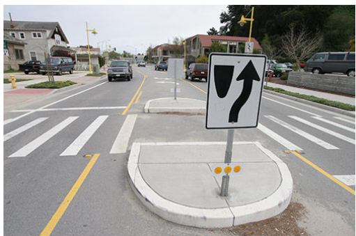
The construction of pedestrian refuge islands (shown at left) can lessen the amount of collisions between pedestrians and motor vehicles at or near dangerous pedestrian crossings along North Lamar Boulevard (right). Photo at left courtesy of: http://www.livablestreets.com/streetswiki/pedestrian-refuge-island
