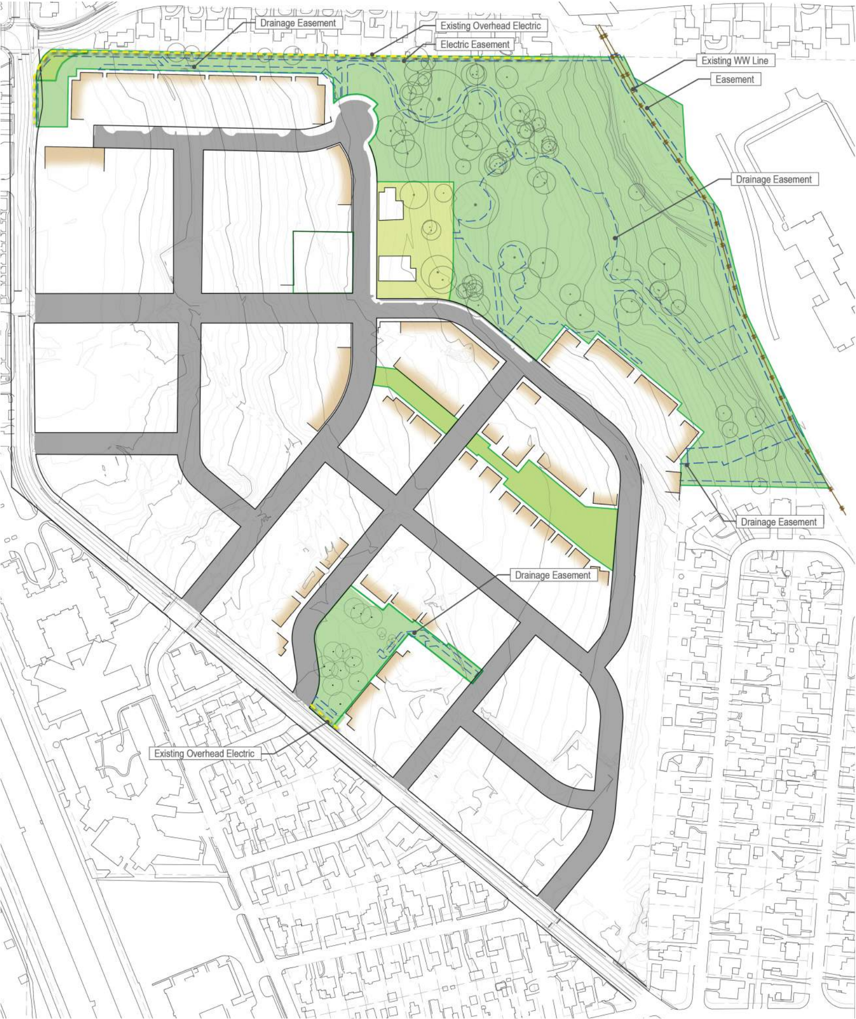
Figure 2 -3: Existing and Proposed Utilities Exhibit
