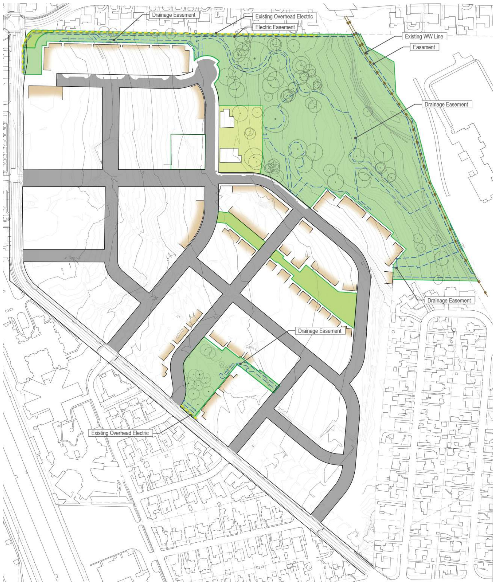
Figure 2 -3: Existing and Proposed Utilities Exhibit
