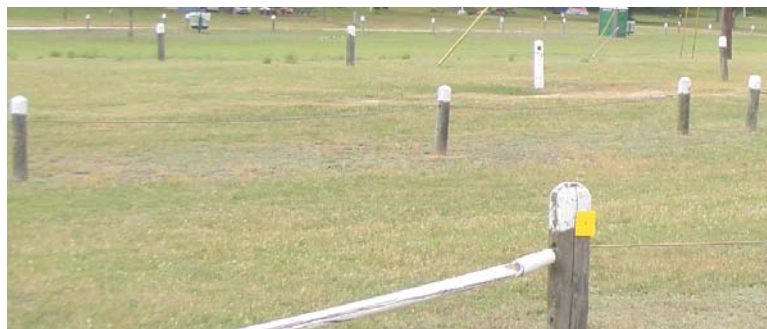
Bollard-and-Cable System for Parking Delineation
