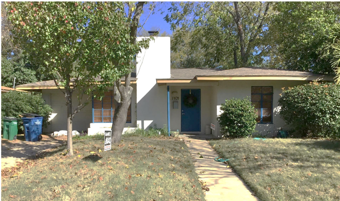
Figure 29. A Minimal Ranch house at 1404 Bentwood Road constructed in 1948 (Survey ID 215045_01). This house, like many others in the Delwood II neighborhood, was constructed of concrete block walls and clad in stucco, which was uncommon in Austin. The smooth walls, along with features like the corner windows, low-pitched roof,
