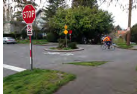
Stop sign oriented to traffic crossing a neighborhood bikeway
