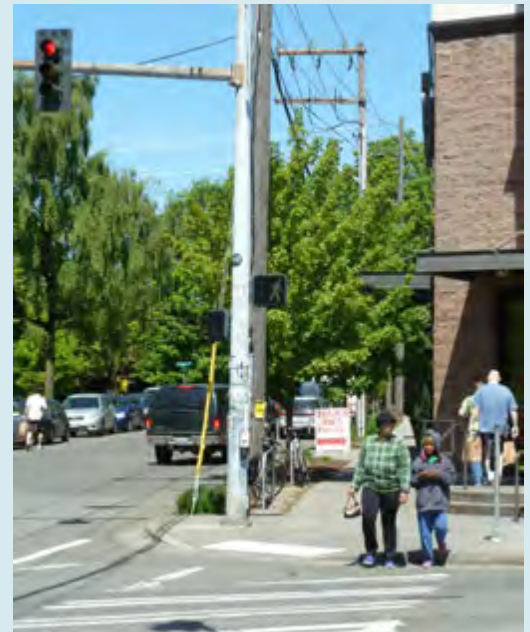
With a Leading Pedestrian Interval, motorists have a red signal for the first 3-5 seconds of the WALK phase.
