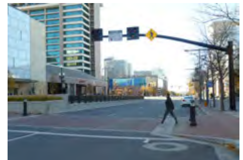
Pedestrian hybrid beacon on a downtown street
