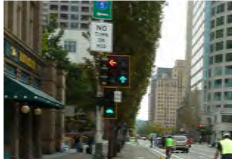
Reflective back plate makes the signal more visible
