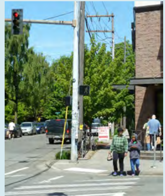
With a Leading Pedestrian Interval, motorists have a red signal for the first 3-5 seconds of the WALK phase.
