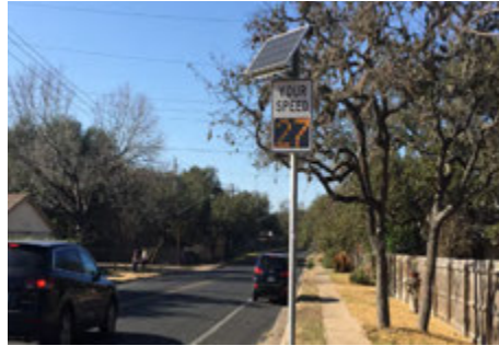
Solar-powered speed radar sign
