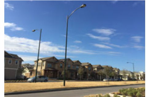
Cobra style lights illuminate the street, but not the pedestrian realm
