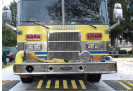
Speed cushions allow for larger vehicles such as fire trucks to pass through unimpeded
