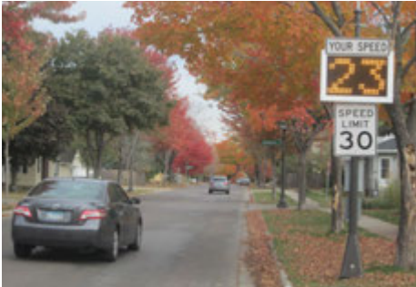
Speed feedback sign displays a driver's speed compared to the speed limit
