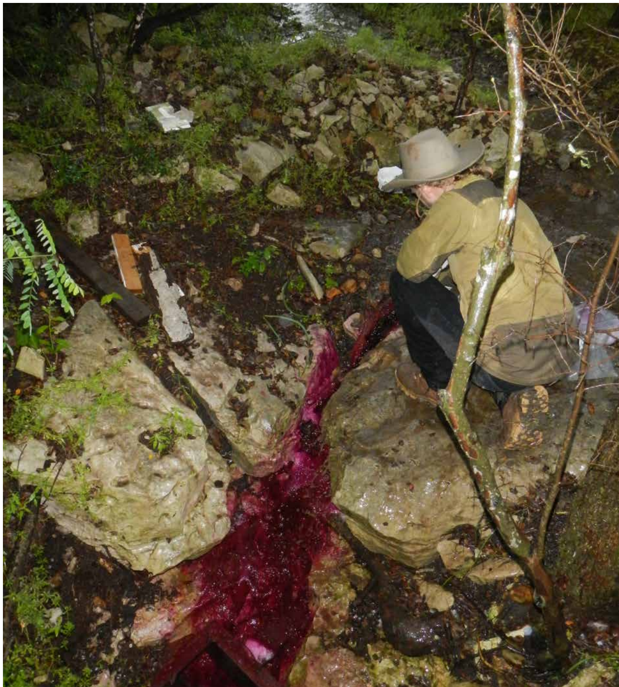
Dye injection in cave at the intersection of MoPac and SH45SW. This dye was not detected in Flint Ridge Cave but was detected more than 9 miles away in Barton Springs.
