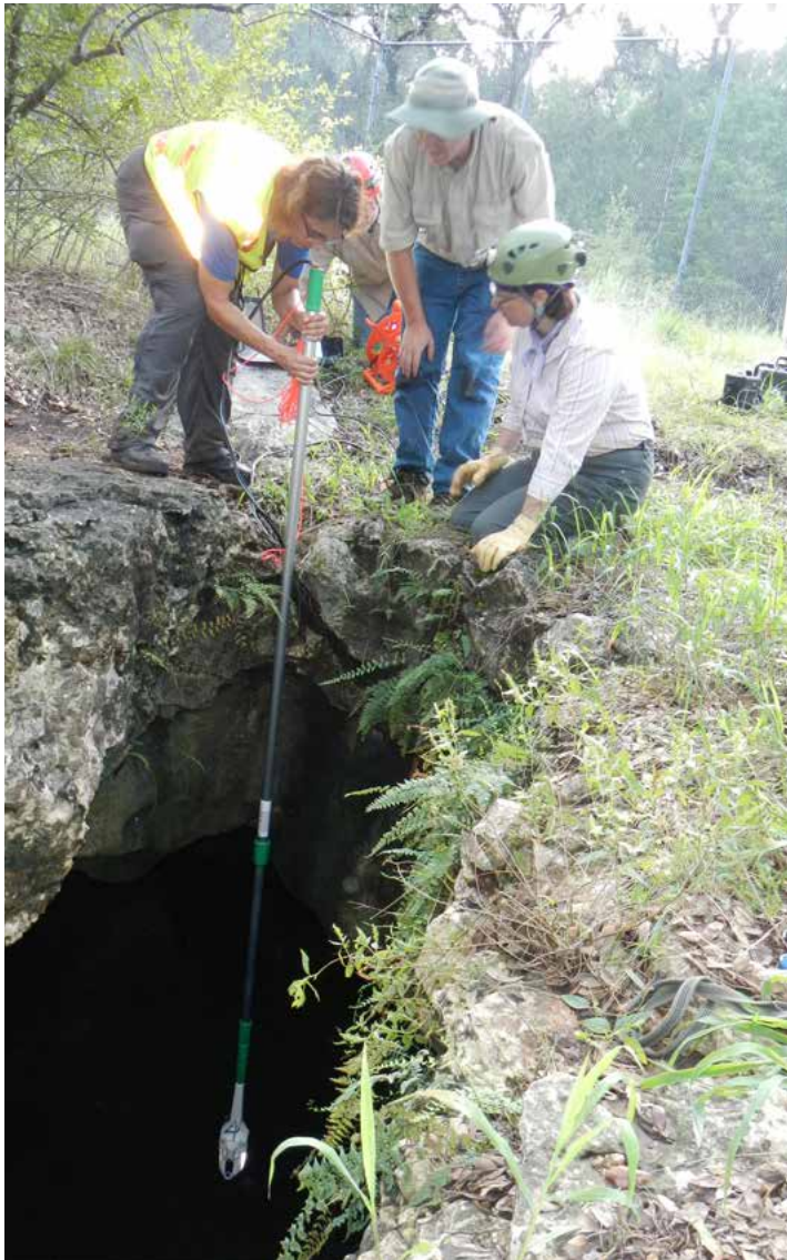
The LIDAR void inspection tool being tested in the Goat Cave Karst Preserve
