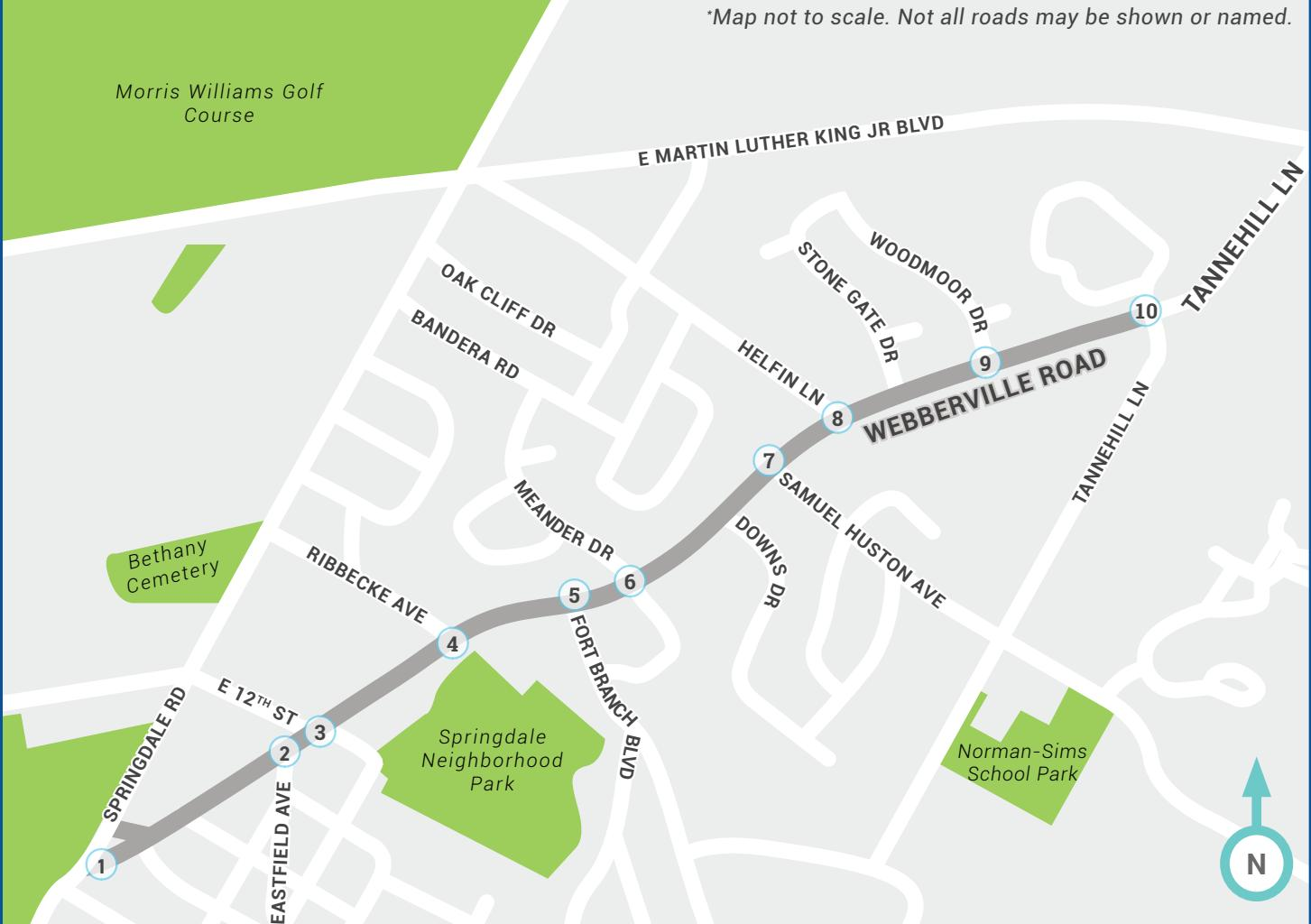
All numbered intersections will have new or rebuilt Americans with Disabilities Act (ADA)-compliant curb ramps. Eastfield Avenue, East 12<sup>th</sup> Street, and Helfin Lane intersections will also be realigned. The realignment will "square up" the intersection by aligning the roads approaching the intersection so they are no longer at an angle. The realignment will reduce motor vehicle speeds, shorten pedestrian crossings, and improve visibility for all users.
