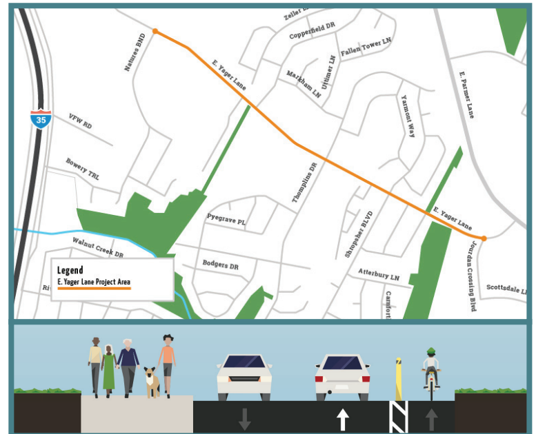
Typical cross section view of East Yager Ln. planned changes showing a shared use pathway on the south curb and a protected bike lane on the north curb. Draft design only. Final improvements may look different due to project enhancements
