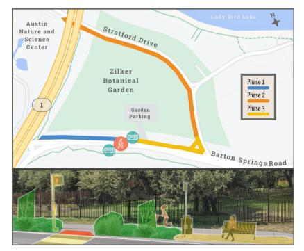
Top: illustrated aerial map\* of the project limits and construction phases. Bottom: rendering of the new shared use path, pedestrian crossing, and bus stop on Barton Springs Drive, facing north. \*Map is not drawn to scale or intended to be used for engineering purposes.
